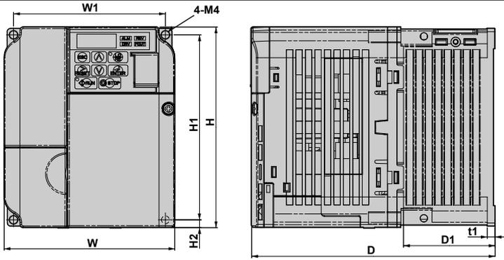
The figure shows two mechanical drawings of the Yaskawa AC Drive. The left drawing is a front view showing the drive's face with various terminals and labels. Dimensions W1, W, H, H1, and H2 are indicated. A 4-M4 screw is shown at the top right. The right drawing is a side view showing the drive's profile and cooling fins. Dimensions D, D1, and t1 are indicated.
