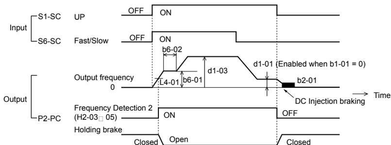
**Figure 4.7 Holding Brake Time Chart**
