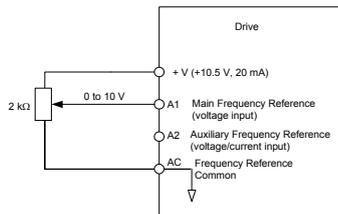
Figure 4.8 Voltage Input for the Main Frequency Reference
