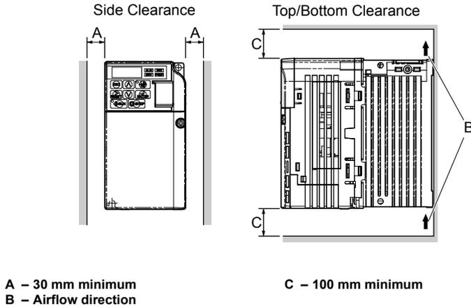
Figure 2.2 Correct Installation Spacing
