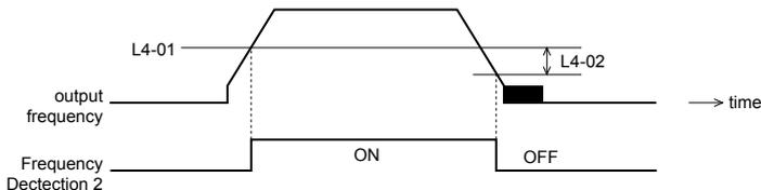
Figure 4.6 Frequency Detection 2
