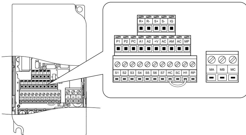
Figure 3.5 Removable Control Circuit Terminal Block
