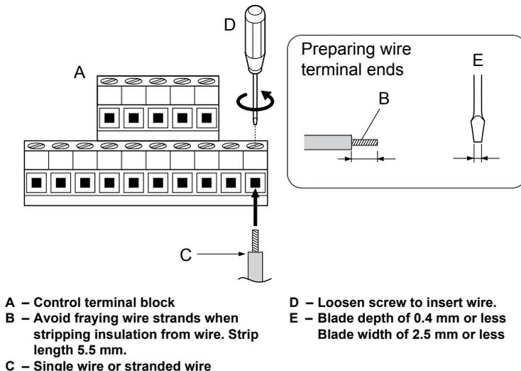
**Figure 3.7 Terminal Board Wiring Guide**
