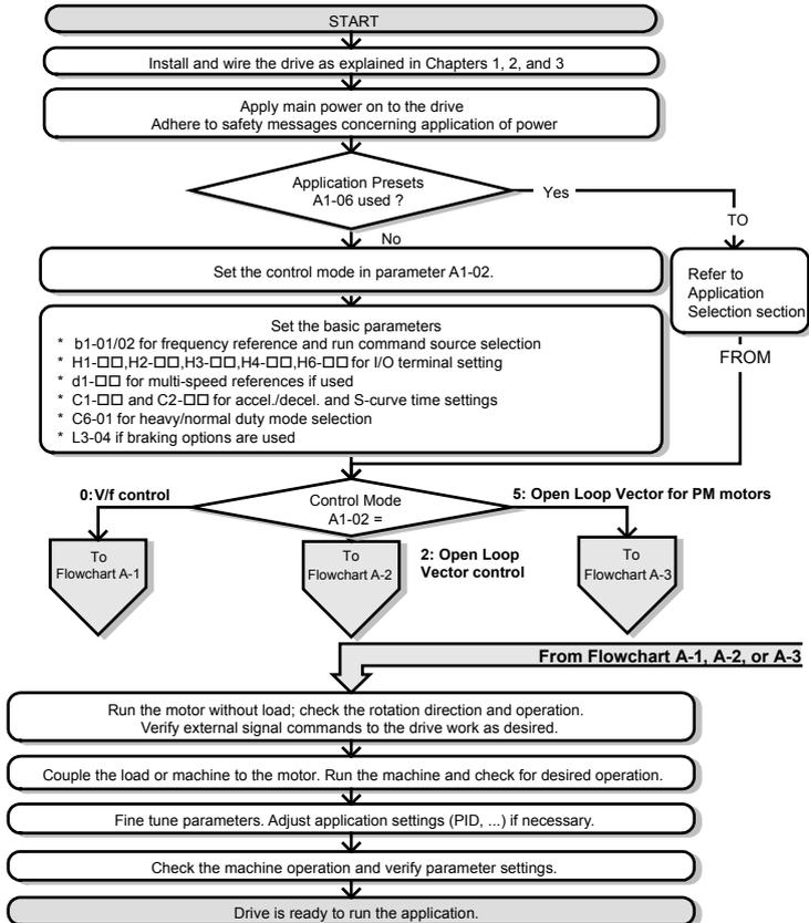
**Figure 4.2 Basic Start-Up and Motor Tuning**
